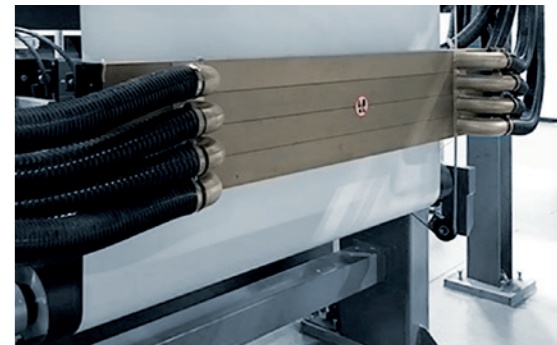
web cleaner installed in a laminator
