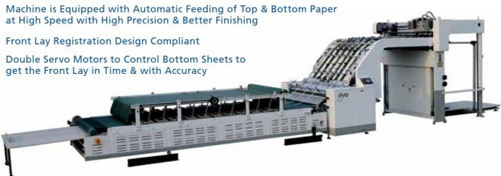
Appropriate paper: Top sheet 200-450g, Bottom sheet +250g A/B/C/E/F flutes Speed: 5500-6000 sheets / hour Sizes from 1300\*1100 to 1600\*1400mm.
