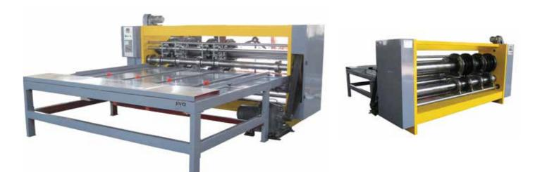
**Cutting & Slotting** Creasing & Edge Cutting of Blanks in Single Operation
