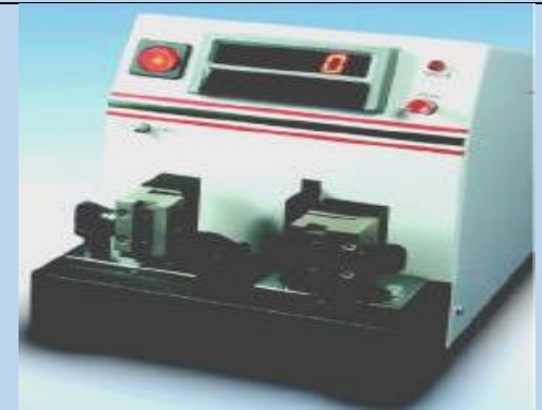
Crease & Board Stiffness Tester (GEC-P40411)
